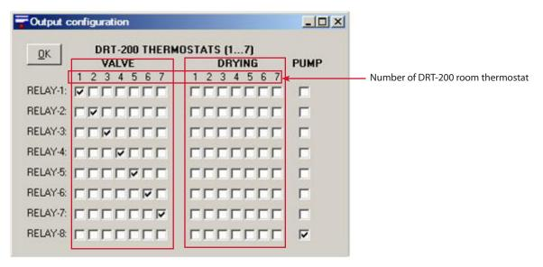
Groups are define the functions (Valve -Actuator-, Drying –Dehumidifier-, Pump)
