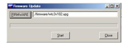
When the Laptop is connected to the WTC-3 and the connection is established then you can "Start" the software update. The program automatically replaces the software for the new one and keeps all settings.
