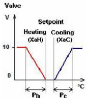
The proportional regulation parameters are fixed in the software! According to the result of dew point c alculation the WTC will regulate the mixing valve with 0-10 V. (0V- fully closed , 10V- fully open)
