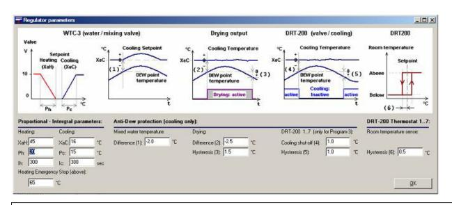
Heating set point XaH: XaC: Cooling set point Ph: Proportional parameter for heating (fixed) lh: Integral parameter for heating (fixed) Pc: Proportional parameter for cooling (fixed) Integral parameter for cooling (fixed) lc: Difference (1) for mixing valve:
