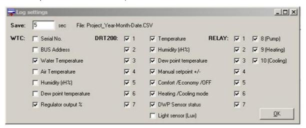
Can be set the saving time interval in second and all requested data what you want to record. To start the logging function just checked the Log box on the main panel and the recording starting automatically according to the setting. This function automatically create an "csv" extract file in the Project\_2010-10-13
