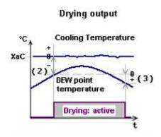
If the CHC system is installed with mixing valve and drying unit (dehumidifier) then the base unit can control the humidity in the room beside of the proportional regulation. With the software you can set 2 control parameters.
