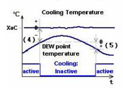
DRT-200 measuring the room temperature and relative humidity. WTC-3 can calculate from these data the dew point value. With the software you can set two control parameters.
