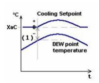
If the CHC system is installed with mixing valve then the control will be much more accurate thanks to the proportional regulation of WTC-3.
